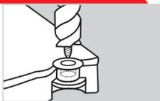
If a service tool is not available, the clenched head of the rivet may be removed by drilling or chiselling. [Extreme care must be taken to ensure the brake shoe rivet holes are not damaged during this operation].
